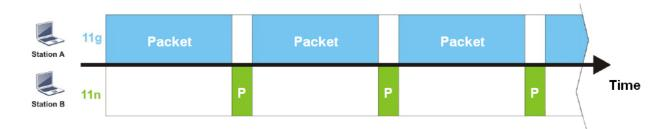
To improve this problem, Airtime Fairness is added for VigorAP 902. Airtime Fairness function tries to assign *similar airtime* to each station (A/B) by controlling TX traffic. In the following figure, Station B(11n) has higher probability to send data packets than Station A(11g). By this way, Station B(fast rate) gets fair airtime and it's speed is not limited by Station A(slow rate).
