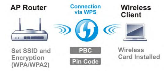
It is the simplest way to build connection between wireless network clients and VigorAP 902. Users do not need to select any encryption mode and type any long encryption passphrase to setup a wireless client every time. He/she only needs to press a button on wireless client, and WPS will connect for client and VigorAP 902 automatically.
