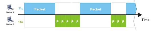
It is similar to automatic Bandwidth Limit. The dynamic bandwidth limit of each station depends on instant active station number and airtime assignment. Please note that Airtime Fairness of 2.4GHz and 5GHz are independent. But stations of different SSIDs function together, because they all use the same wireless channel. IN SPECIFIC ENVIRONMENTS, this function can reduce the bad influence of slow wireless devices and improve the overall wireless performance.
