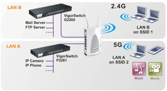
In the above figure, VigorAP 902 is used to control the wireless network connection. It can separate the wireless traffic between accessing internal server and the usage of video. Wireless station connecting to VigorAP 902 with SSID 2 can get the IP address with the network segment of 192.168.1.0/24 (LAN-A); wireless station connecting to VigorAP 902 with SSID 1 can get the IP address with the same network segment of 192.168.2.0/24 (LAN-B).
